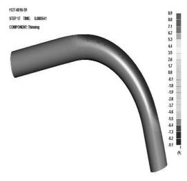
壁厚减薄率 $(R_b = 4D_n, \theta = 90^\circ)$
